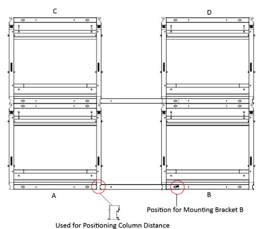
Figure 2-3 Determine Mounting Position for Bracket B
