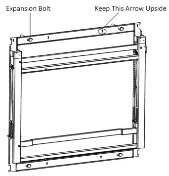
Figure 2-1 Secure the Bracket
