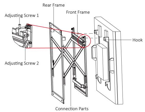
Figure 2-6 Mount Displays to Brackets
