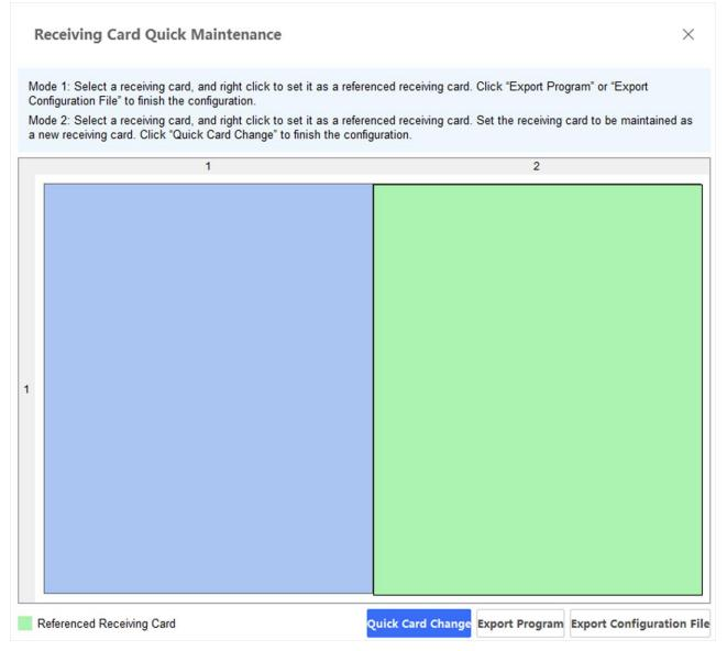
Figure 4-14 Receiving Card Quick Maintenance
