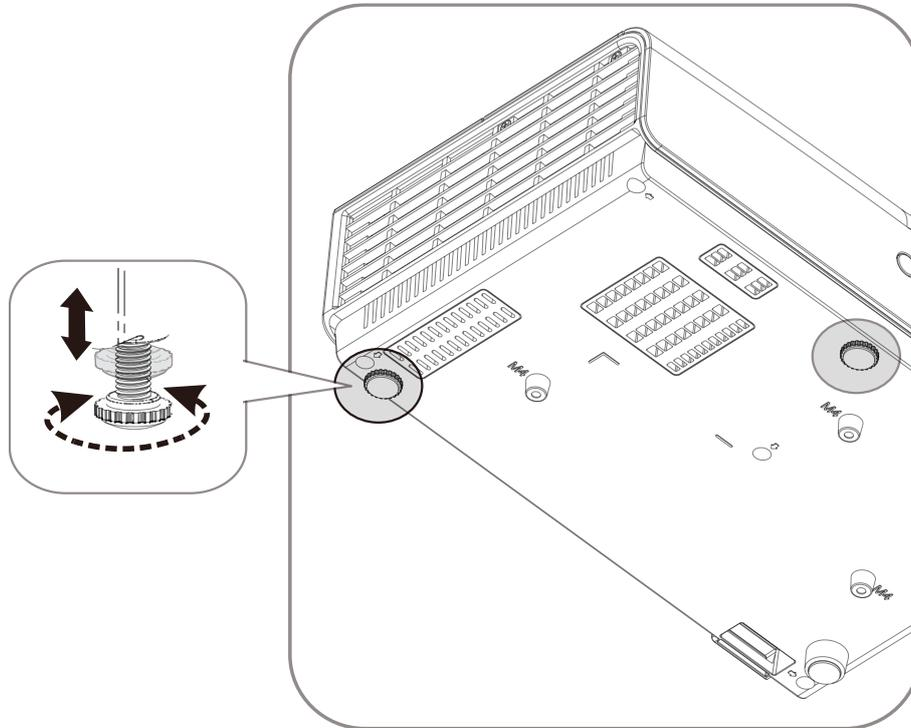
To adjust the angle of the picture, turn the tilt-adjuster right or left until the desired angle has been achieved.
