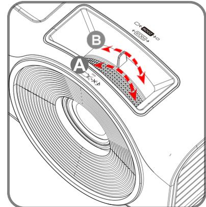
2. Use the **Image-focus** control (on the projector only) to sharpen the projected image **A**.
