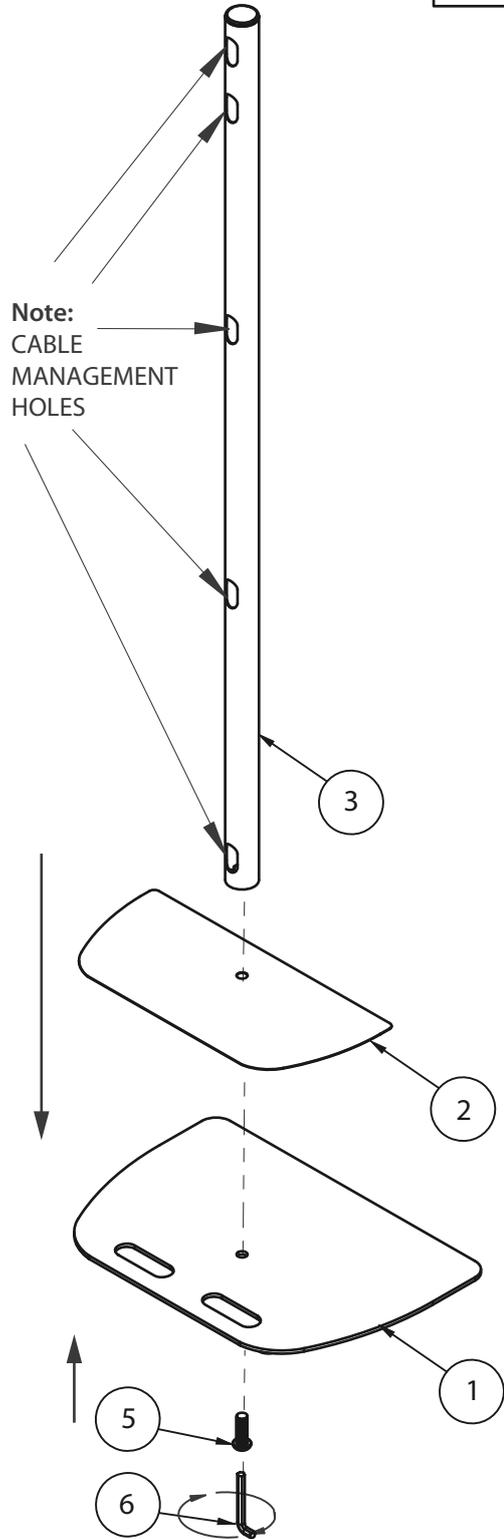
Note: Position pole so the cable management holes face the rear of the stand.
