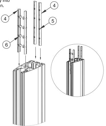
Join the columns together by sliding the 60cm column (part 1) onto the connector bars (part 4).
