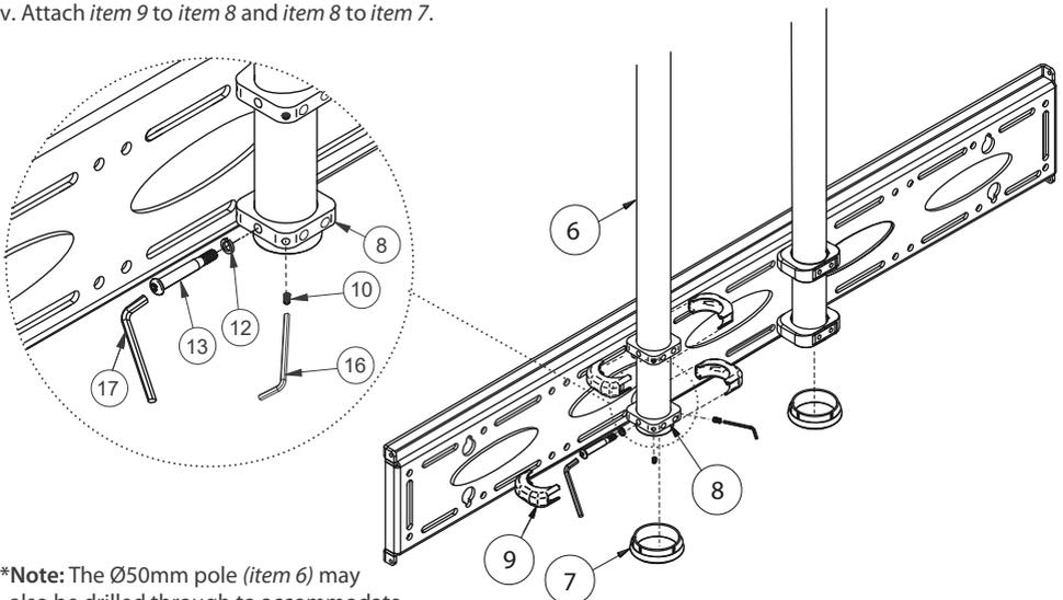
\*Note: The Ø50mm pole (*item 6*) may also be drilled through to accommodate the safety screw (*item 13*).
