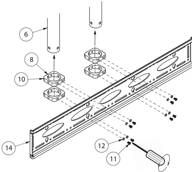
iii. Once positioned on *item 6*, tighten *item 10* on the back of *item 8*.
