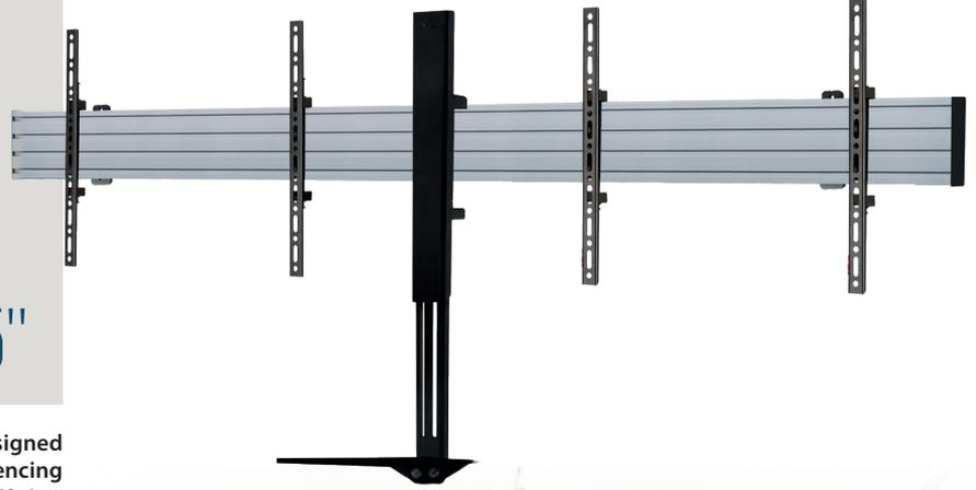
BT8416 is a premium wall mounting solution designed to mount two screens side by side for video conferencing applications. The mount features an adjustable VC shelf that gives the user the flexibility of mounting a VC camera above or below the screens. Additional features include adjustable levelling screws for easy height adjustment of the screen once mounted, cable management clips and safety screws that help to prevent un-authorised removal of the screen.
