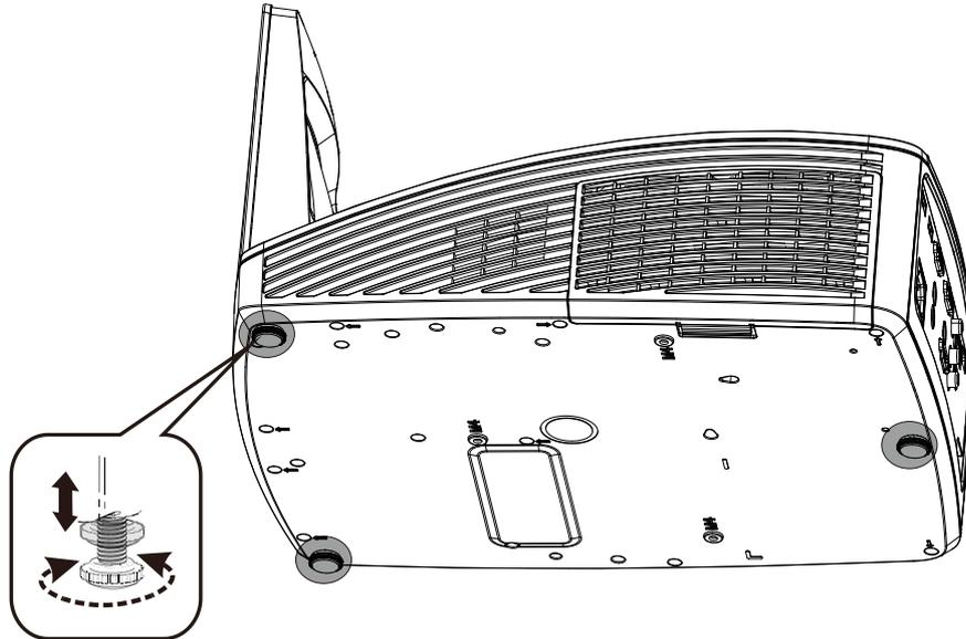
To adjust the angle of the picture, turn the tilt-adjuster right or left until the desired angle has been achieved.
