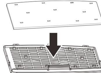
4. Replace the filter cover back to the projector by pushing gently in the direction shown.
