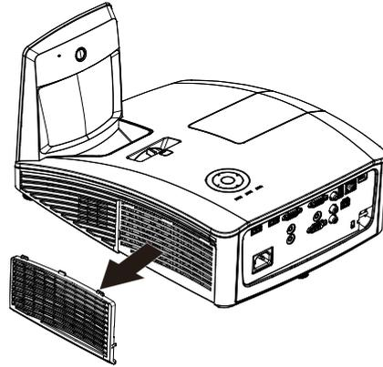
2. Or lift the filter from the filter cover.
