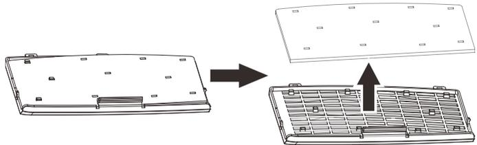
3. Replace a new filter module or replace filter into cover.
