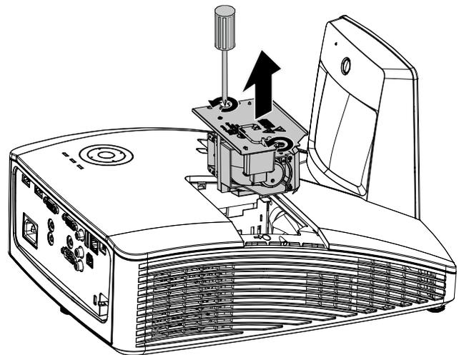
6. Reverse steps 1 to 5 to install the new lamp module. While installing, align the lamp module with the connector and ensure it is level to avoid damage.
