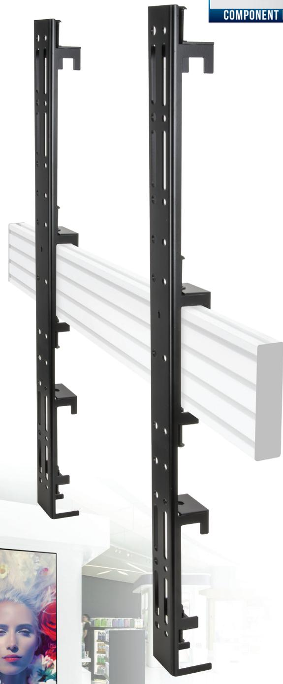
These interface arms are designed to mount XL screens in a fixed position across one or two System X horizontal mounting rails. The universal design is compatible with a variety of different screens and allows them to be mounted in either landscape or portrait orientations. Levelling screws on each interface arm provide post installation height adjustment and a mounted depth of 64mm from the wall allows easy access for cables and connectors.
