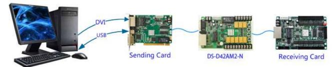
Connect the DS-D42AM2-N between any two receiving cards.
