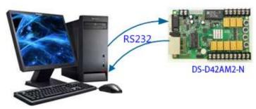
• Connect the DS-D42AM2-N between the first receiving card and the sending card (or independent controller).
