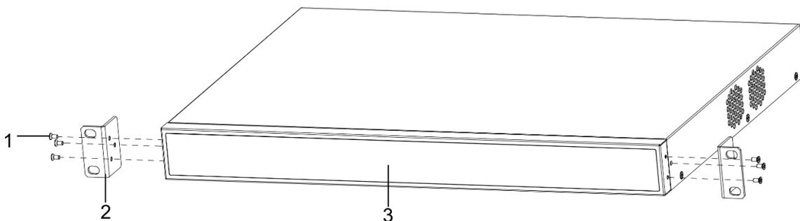
Figure 2-8 Install the Mounting Brackets
