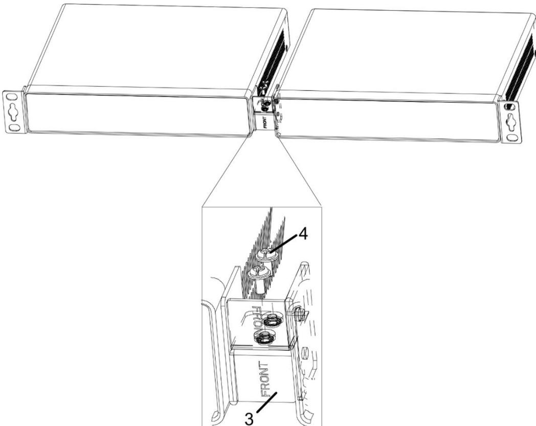
Figure 2-3 Secure the Connecting Brackets 1
