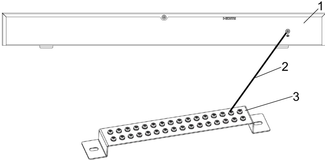
Figure 2-10 Connect the Grounding Cable to the Grounding Bar
