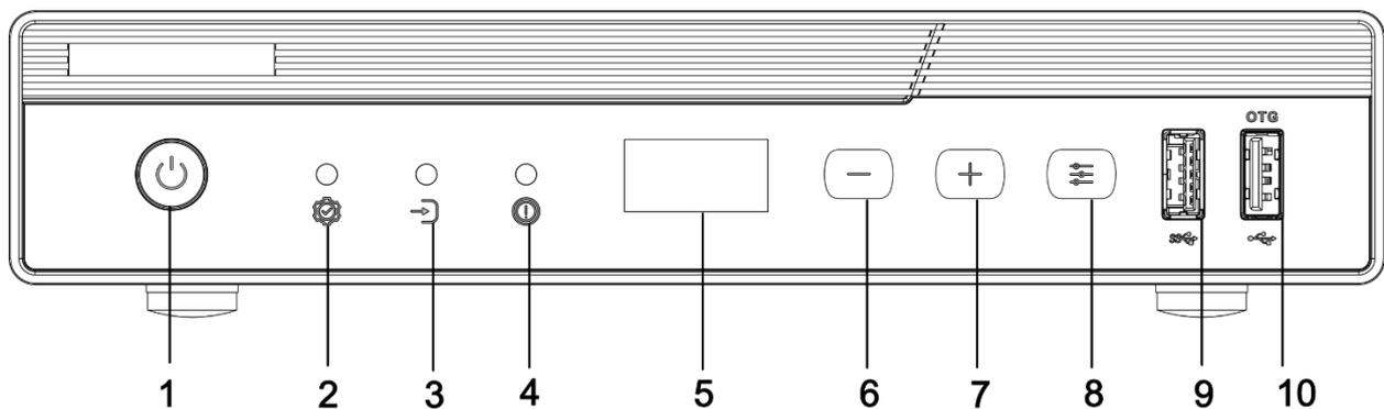
Figure 1-1 Front Panel of 2K Device
