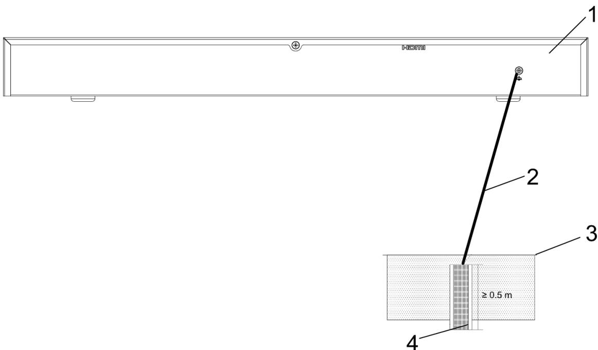
Figure 2-11 Connect the Grounding Cable to the Grounding Electrode
