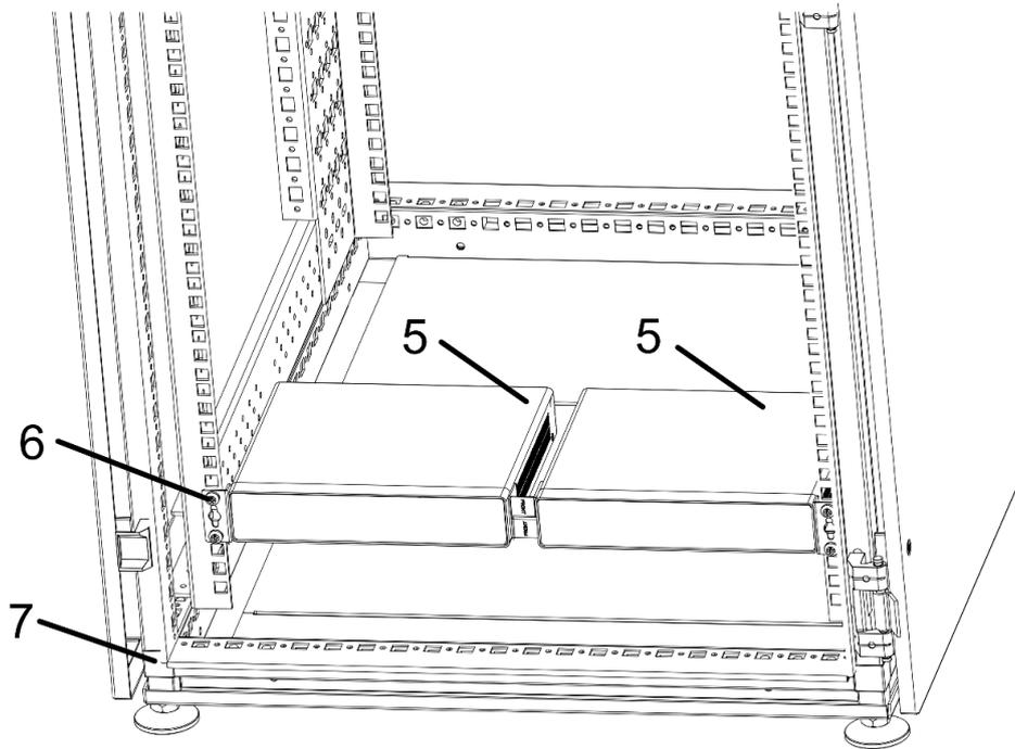
Figure 2-4 Secure Devices to the Rack
