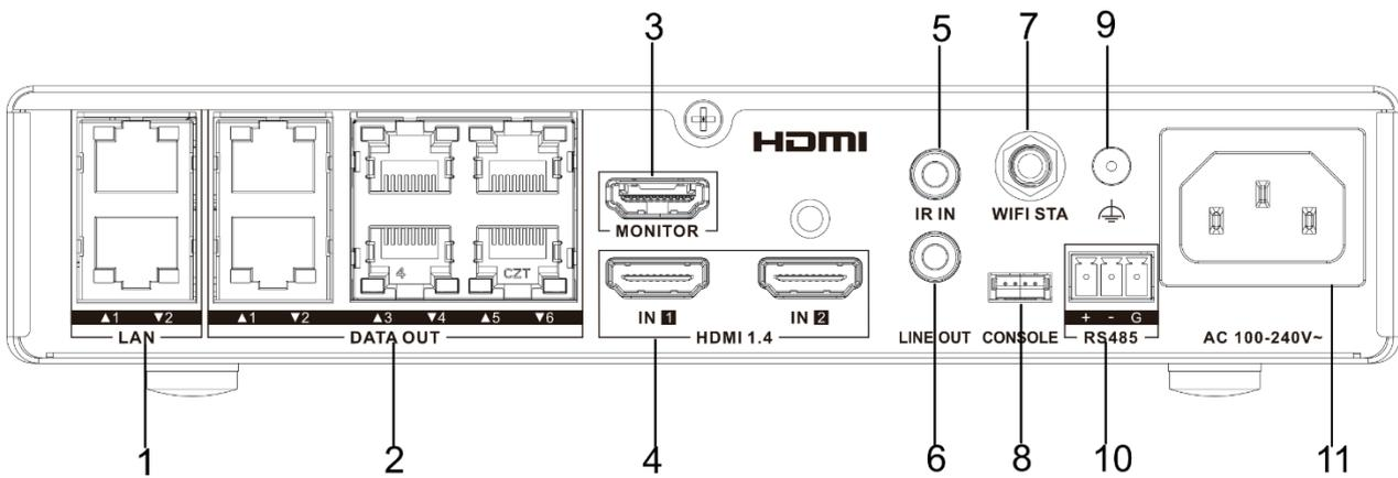
Figure 1-4 Rear Panel of 2K Device with 6 Outputs
