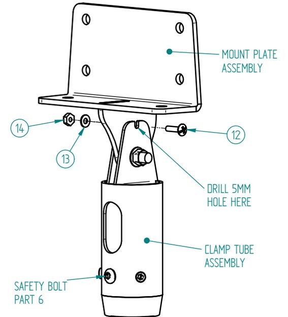
WHEN MOUNTING HEAVY EQUIPMENT AN OPTIONAL LOCKING BOLT (PART 12) MAY BE USED TO SET THE POLE VERTICAL AT ANY CEILING PITCH UP TO 45°
