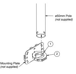
ii) Retro fitting the collar onto the pole - For situations where you cannot hook the collar over the pole. Disassemble the collars by undoing the M6 x 20mm screws (Part 3) with the Allen key (Part 7). Attach mounting plate to front half of collar (Part 1)\*.
