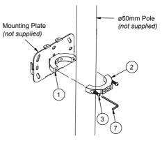
\* It is important to fix the mounting plate to the front half of the collar (Part 1) so you have access to the M6 x 20mm screws. **Note:** Mounting plates can be attached to the collar after the collar is fixed onto the pole.
