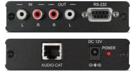
The PU-305BDA-TX is an analogue Stereo over CAT5e/6/7 Transmitter which can send and receive analogue audio signals over a single run of CAT5e/6 cable up to 300m. It has the added benefit of RS-232 pass-through allowing control of devices and the Power over Ethernet (PoE) function can power the receiver unit eliminating the need for a second power supply. As the unit has bi-directional capabilities, this device can also receive audio signals back from the connected receiver.
