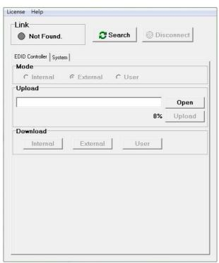
Connect the unit under power ON status with USB cable from PC/Laptop. Click on Search to allow the unit to be lined up.
