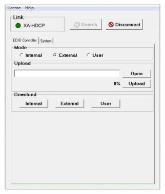
Click on System to learn the unit's Current Firmware version. To update simply open the \*.bin file and click on Update. Once the update is finished click on Disconnect and re-power on the unit will complete the update procedure.
