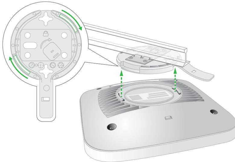
8. Twist the AP clockwise to lock it onto the mounting plate.
