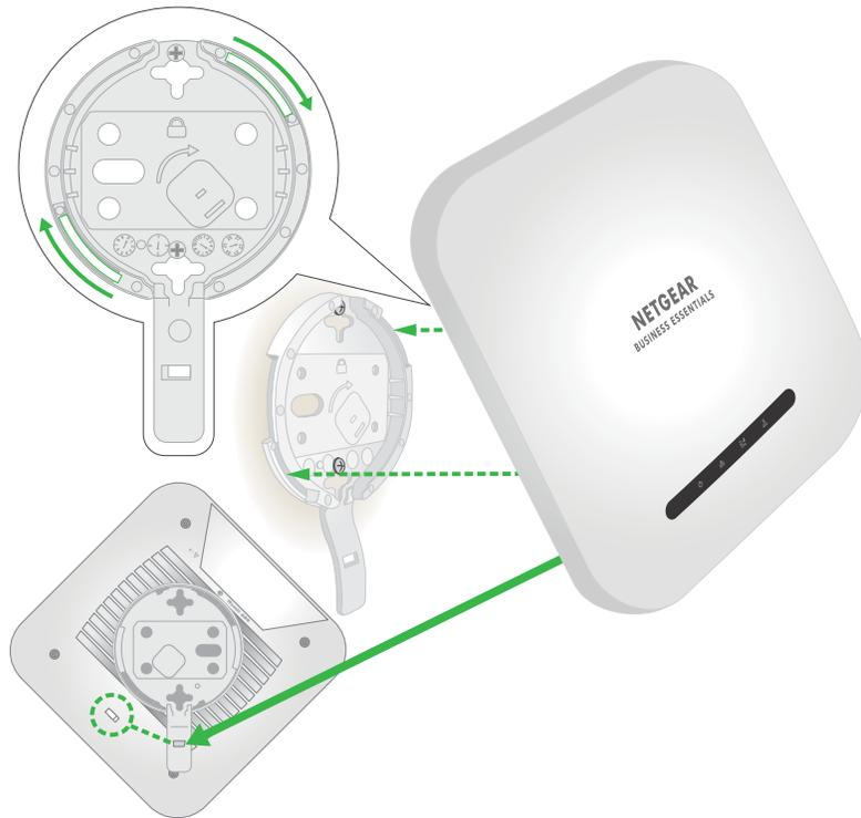
8. Twist the AP clockwise to lock it onto the mounting plate.
