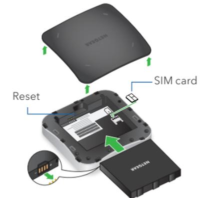
5. Align the battery connectors and insert the battery making sure the contact side of the battery goes under the two plastic tabs in the battery recess.
