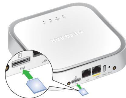
3. Gently insert the nano SIM card into the nano SIM card slot.
