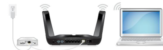
The router now uses the LM1200 modem's LTE network as its main (primary) Internet connection.
