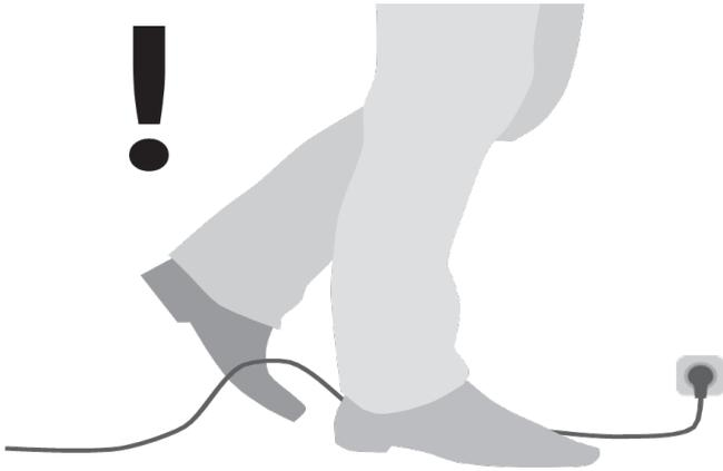
Make sure the power cable is not placed in a walking route to prevent potential trip hazards.
