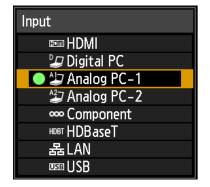
The currently active input signal is marked with a green circle and enclosed by a orange border.
