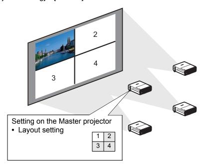
If the image does not switch to the image for the corresponding number, adjust the IP address setting.
