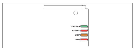
The projector status is shown by the LED indicators (off / lit / flashing).
