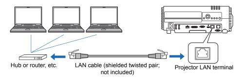
When using the HDBaseT port, connect the projector as follows.
