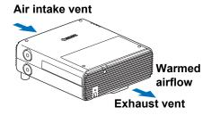
ventilated location. (Ensure a minimum clearance of 50 cm (1.6 ft.) above, on both sides, and behind the projector, as shown below.)
