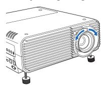
To adjust the image size, turn the lever on the projection lens. Change the projector installation position (P42) if your desired image is too large or too small to adjust it with the zoom function.
