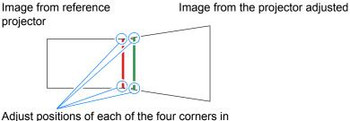
the overlapping area. Correcting the position of one point will also move the point on the opposite side of the overlapping area, so that the screen as a whole is corrected.
