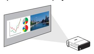
Splits the screen for projection of two separate input signals at once. (P157)
