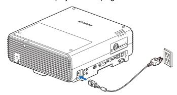
• Be sure to connect the ground wire of the power cord to ground.
