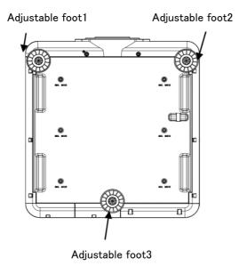
The figure on the left is a schematic diagram of the bottom of the projector.
