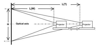
Picture of the height (H) is projected at between the shortest distance L(W) and L(T).
