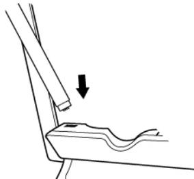
6. Connect the other end of the connector bar to the MimioTeach bar as shown.
