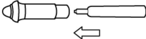
6. Align the arrow on the pen body with the arrow on the top part of the pen.
