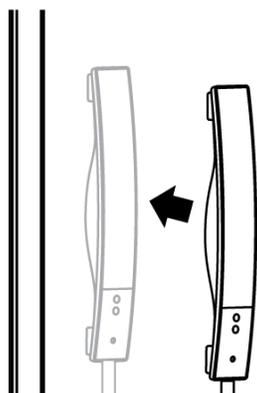
The MimioTeach bar attaches securely to any magnetic whiteboard. See [Mounting MimioTeach to a Non-Magnetic Whiteboard](#) for information about mounting the bar to a non-magnetic whiteboard.
