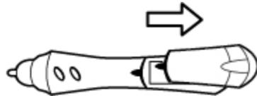
2. Insert one AA battery into the battery compartment.
