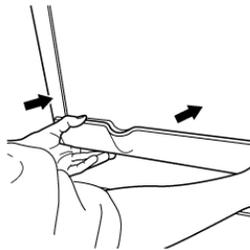
The MimioCapture tray attaches securely to any magnetic whiteboard. See [Mounting MimioCapture to a Non-Magnetic Whiteboard](#) for information about mounting the tray to a non-magnetic whiteboard.
