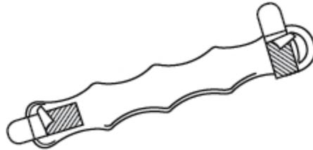
2. Hold the Mimio Capture Kit pen holder vertically, and press firmly against the whiteboard as shown.
