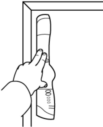
The Mimio Interactive bar attaches to any whiteboard using the suction cups on the back of the bar.
