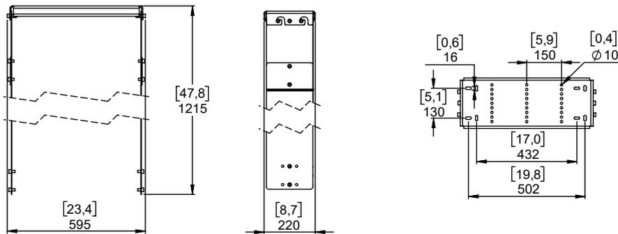
For fixation, you have the choice between M8 and M10 (Fasteners not included)
