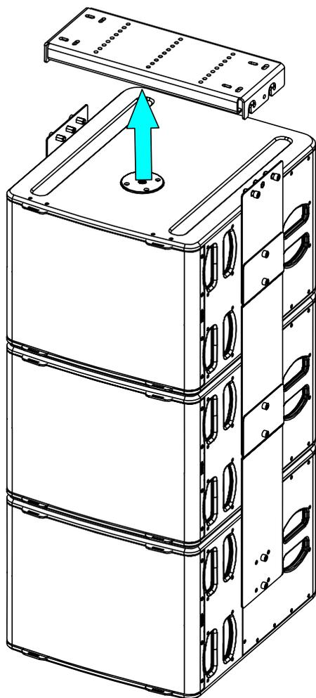
Tighten the screws. Secure with the 2 provided M10x30 screws.
