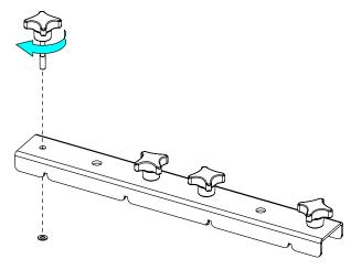
Mounting of a hook on the accessory (fasteners not provided). For 10mm (0.4 inch) diameter fasteners.
