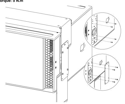
Warning: Use only provided screws (thread lock coated or use Loctite 243).
