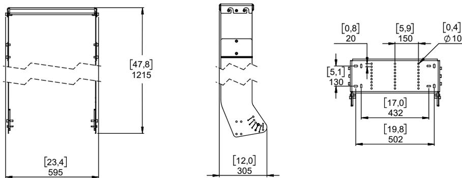
For fixation, you have the choice between M8 and M10 (Fasteners not provided)
