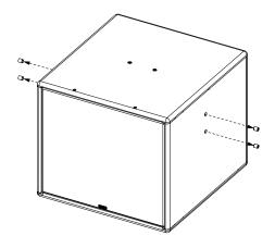
Assemble the Plates on each side of eLS400 using the M10x20 screws.
