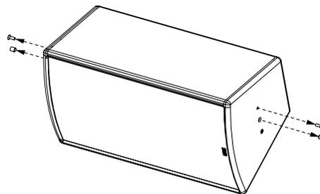
Place ePS10, fasten with M10x20 and M6x25 screws.
