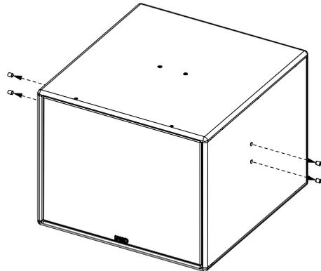
Assemble the Plates on each side of eLS600 using the M10x20 screws.
