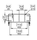
For fixation, you have the choice between M8 and M10 (Fasteners not provided)
