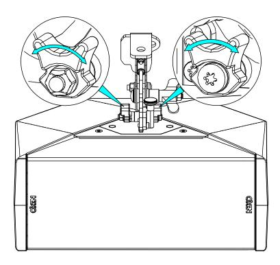
Tilt: Loosen the wing nut to adjust the angle (-45° to +45°).
