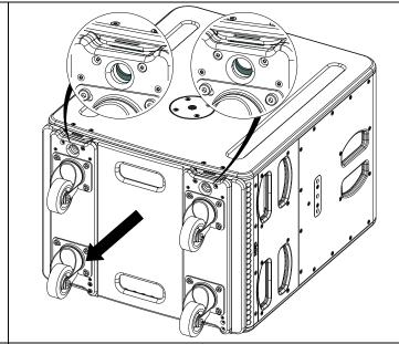
Insert the 2 metal brackets in the spigots.
