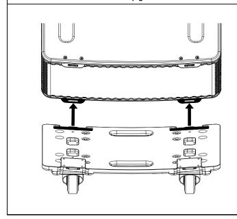
Push the 2 latches and lock the Wheelboard.
